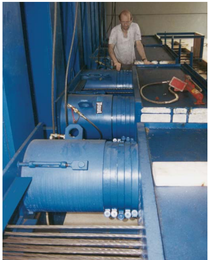
Fig. 1 4 x 8000 kN casting beds with 8 x 4000 kN/225 mm stroke hydraulic cylinders (79–061.10) and 40 support sleeves 4000 kN, 40 mm height (79–020.34)
