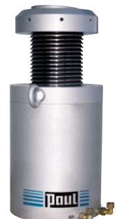
Fig. 14 4000 kN/300 mm stroke threaded-piston cylinder, double acting
