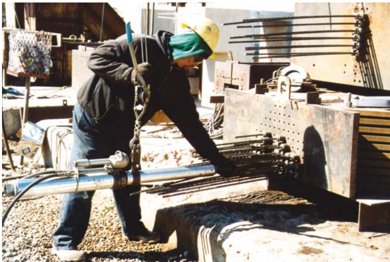
Fig. 7 200 kN two-hose stressing jack, 500 mm stroke at Bayshore Corp., Cape Charles, VA / USA
